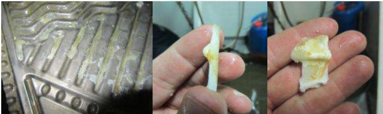
Figure 2. Limescale precipitation on the titanium heat exchanger plates prior to the installation.
