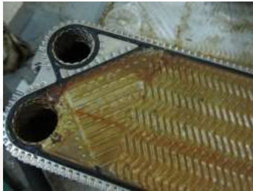
Figure 3. FWG plates while opening covered with slime
