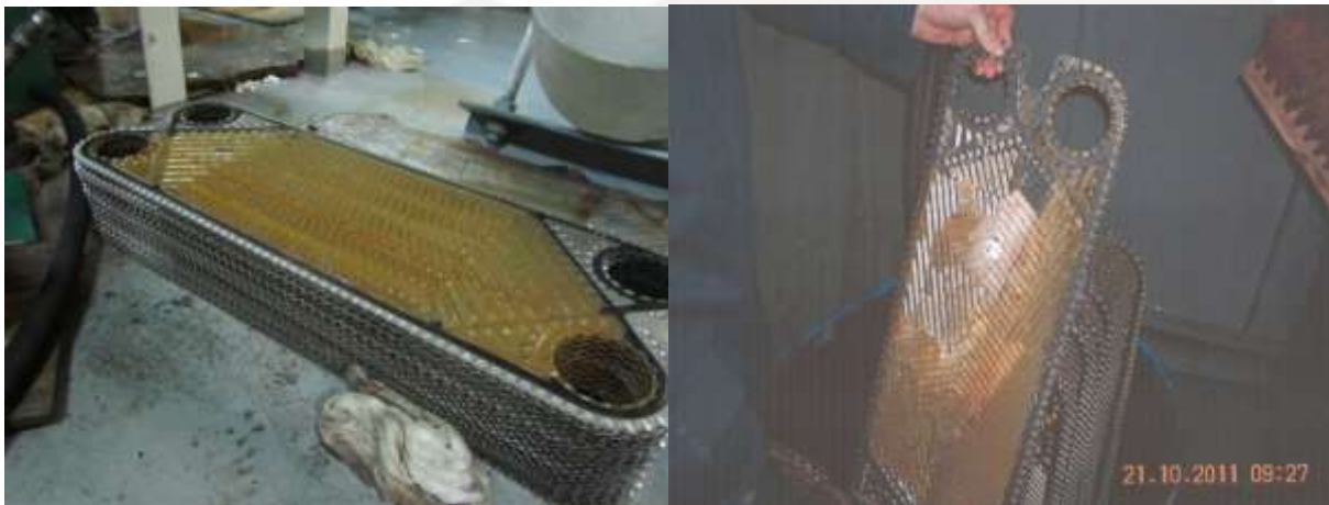
Figure 10. Left: December 2012 – before installation, plates are covered with slime. Right: FWG plates (different FWG unit) treated with chemicals but covered with limescale and slime.
