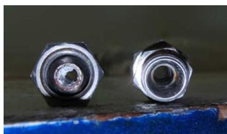
Figure 1 The scaling of an untreated pipe (left) compared to a pipe treated with Hydropath (right) (page 10).
